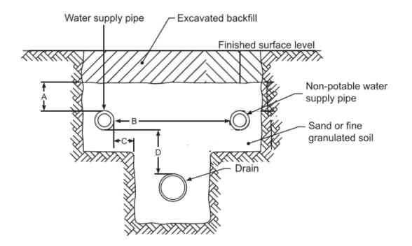
(a) Give the minimum measurement required for each of the distances marked A, B, C and D.
