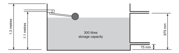
All connection points for the tank are 25 mm.
