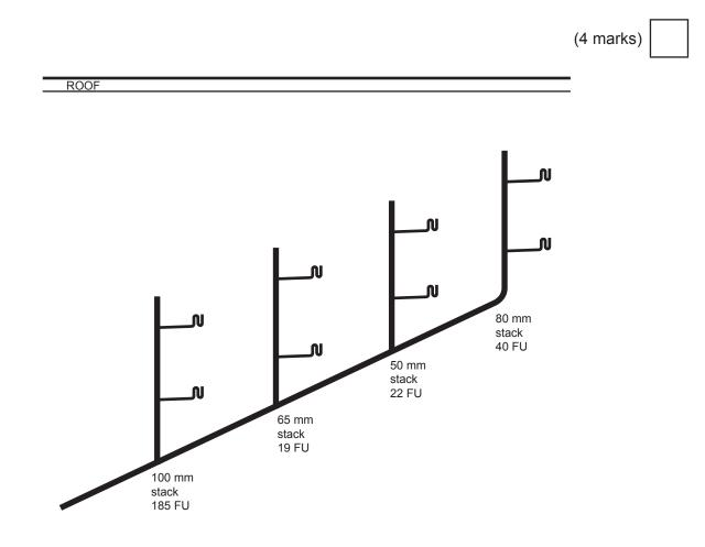
(b) Using the stack diameters and fixture unit ratings (FU) shown on the diagram, size each vent. Write your answers on the diagram.
