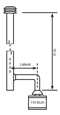
Using the information from the diagram, complete the following tables by giving the minimum size of the flue for each lateral length according to AS/NZS 5601 Part 1.
